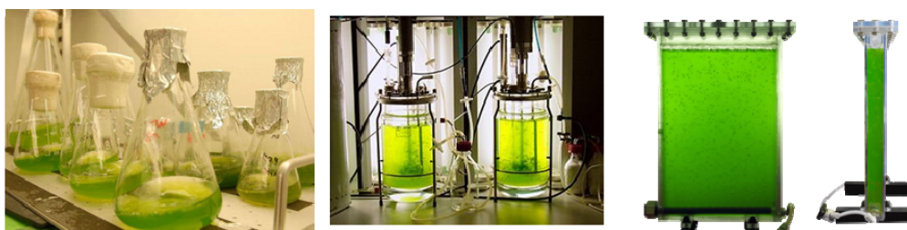
Figure 4 Three examples of contained production of algae: erlenmeyers, fermenters and flat panel reactors
