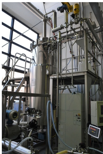
Figure 5 A 1500 litre steel fermenter
